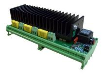
The Power Products range of S3 thyristor power controllers are designed for the control of resistive loads in electric furnaces, and heater batteries in HVAC systems.
