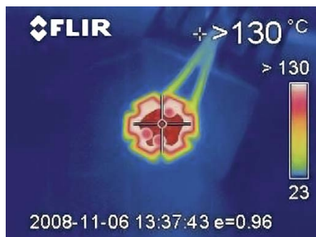
Figure 3: Heat image of an Ostar-LED (4 W), 10 secs. without cooling element
