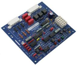
High Current Picket Fence Gate Drive: The transformer-isolated gate drive circuits provide a hard firing initial 13 V open circuit/1.3 A short circuit firing pulse followed by sustaining "back porch" pulses at 6 V open circuit/0.5 A short circuit. The gate pulse burst frequency is 384 times the mains voltage frequency.
